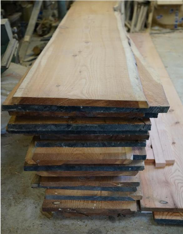
*Figure 2. 30mm thick larch sawn 'through and through' and then kiln dried under restraint.*
