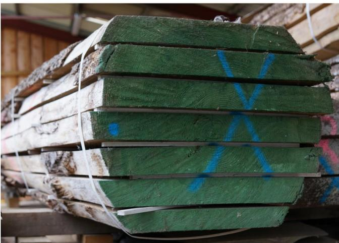
*Figure 1: High grade Welsh grown Douglas fir cut 'through & through' then successfully air dried*
