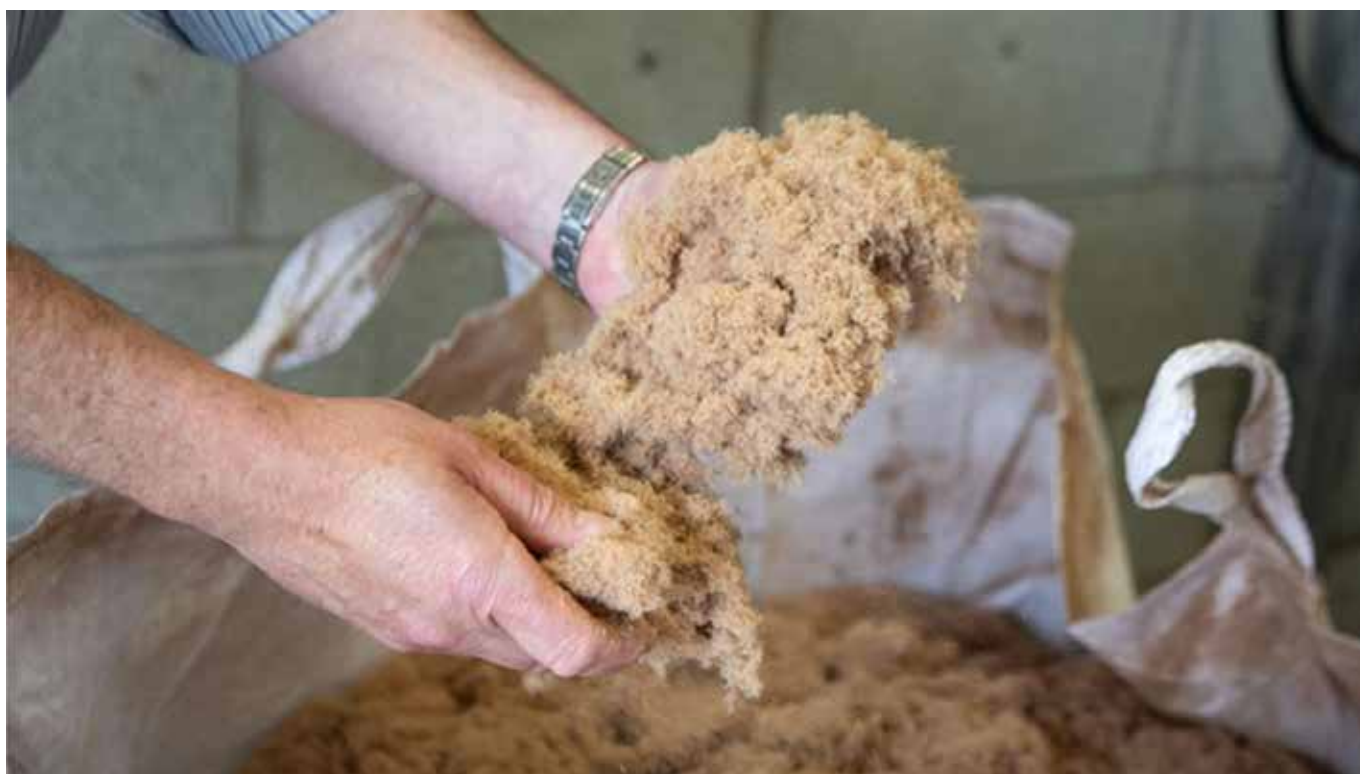
Recycled MDF panel fibres ready for reuse in new MDF panels or wood fibre products such as insulation. Source: MDF Recovery
