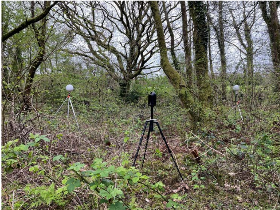
Figure 3. The Leica BLK360 device used to scan a plot (central) and two of the three reference spheres used to act as tie-points to assist in alignment of individual scans.
