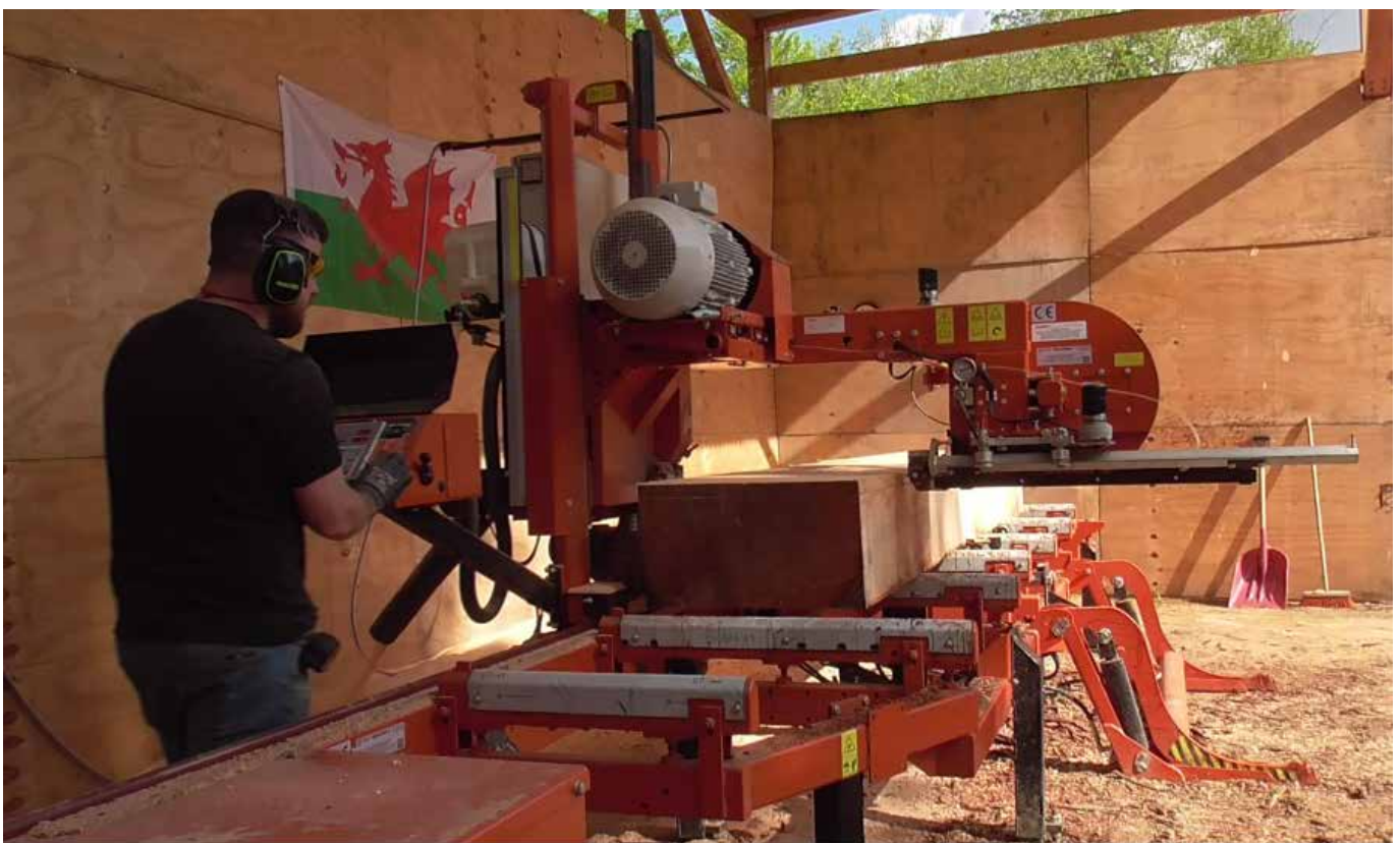
A squared section of Douglas fir being processed into boards at the Signs Workshop
