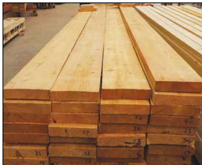
Figure 13: 225mm deep C24 larch from Wentwood forest at Fforest Timber Engineering
