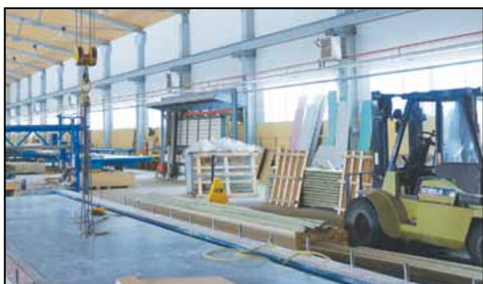
Figure 21: Closed panel production line in Latvia with overhead crane and butterfly tables
