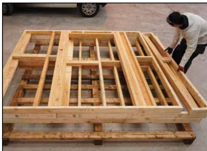
Figure 12: Welsh larch assembled as partly complete open panels at Fforest Timber Engineering
