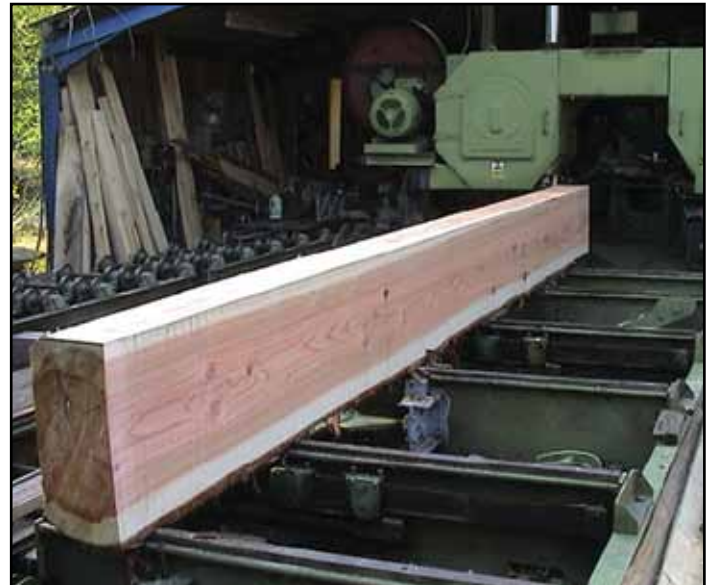
Figure 3: Homegrown coastal redwood being processed at a specialist sawmill in Mid Wales
