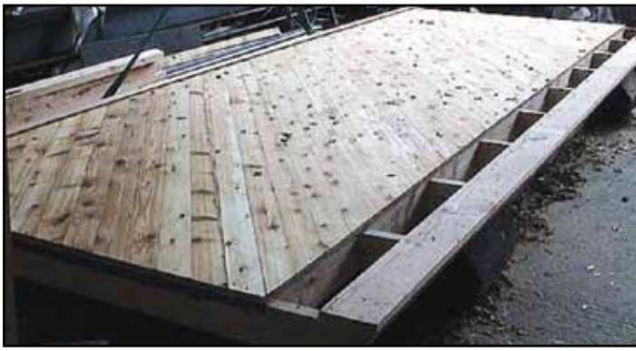
Figure 23: A bespoke 6m. long closed panel made using Welsh Douglas fir and western red cedar
