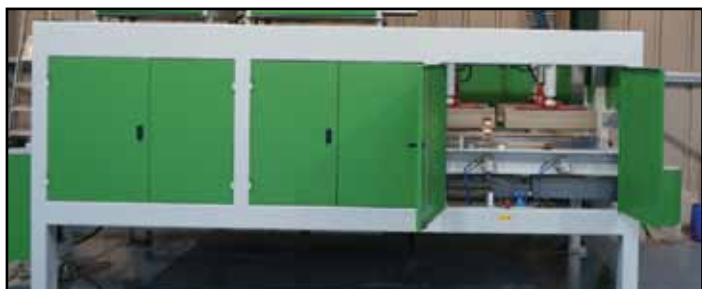
Figure 34: The new radio frequency high volume glulam press at Clifford Jones Timber, Ruthin
